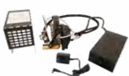
EPK-2V(P)-TR 110V Electronic Valve Kit • 110V electronic valve kit with intermittent pilot ignition • Variable flame height control via remote • AC power operation • Max BTU input: 120,000 (NG) / 180,000 (LP) • Compatible with G4, G45, & G45-2 listed burners • Includes: Variable remote, receiver, and high capacity transformer
