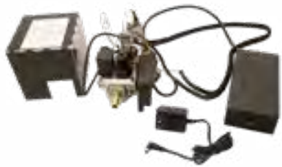
EPK-3V(P)-TR High Capacity, 110V Electronic Valve Kit • 110V electronic valve kit with intermittent pilot ignition • Variable flame height control via remote • AC power operation • Max BTU input: 200,000 (NG) / 320,000 (LP) • Compatible with G4, G45, & G45-2 listed burners • Includes: Variable remote, receiver, and high capacity transformer
