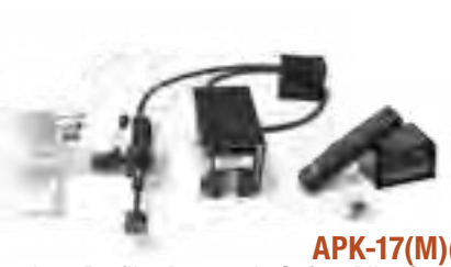
APK-17(M)(P) Low Profile, Automatic Safety Pilot System • Low profile safety valve with standing pilot • Manual on/off switch (optional remote control available) • Variable flame-height control (manual or with remote) • Includes triple heat shield to keep the valve cooler • Max BTU input: 100,000 (NG) / 200,000 (LP) • Compatible with G4, G45, G45-2, & P listed burners • APK-17 & APK-17P models include VR1A variable remote and receiver
