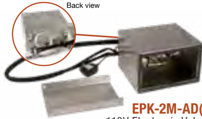
EPK-2M-AD(LP) 110V Electronic Valve Kit • Non-standing flame-sensing pilot • On/off manual operation (wall switch sold separately) • AC power operation • Max BTU input: 88,000 (NG) / 110,000 (LP) • Compatible with G4, G45, G45-2, & PB listed burners
