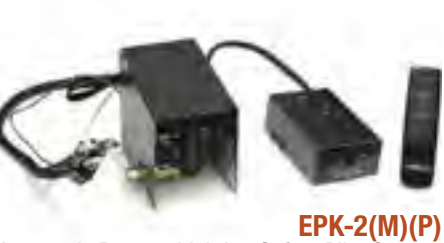
EPK-2(M)(P) Automatic Remote Lighting Safety Pilot System • Intermittent pilot ignition • Non-standing flame-sensing pilot • Manual on/off switch (optional remote control available) • Max BTU input: 120,000 (NG) / 190,000 (LP) • Compatible with G4, G45, G45-2, & P listed burners • EPK-2 & EPK-2P models include RR1A on/off remote and receiver
