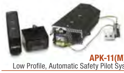
APK-11(M)(P) Low Profile, Automatic Safety Pilot System • Low profile safety valve with standing pilot • Manual on/off switch (optional remote control available) • Max BTU input: 70,000 (NG) / 110,000 (LP) • Compatible with G4, G45, G45-2, & P listed burners • APK-11 & APK-11P models include RR1A on/off remote and receiver
