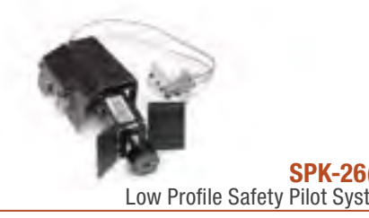
SPK-26(P) Low Profile Safety Pilot System • Low profile safety valve with standing pilot • Includes double heat shield to keep the valve cooler • Max BTU input: 115,000 (NG) / 186,000 (LP) • Compatible with G4, G45, G45-2, & P listed burners
