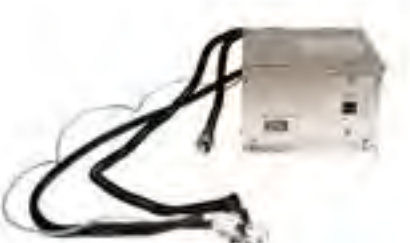
EPK-5(P) AC Powered Electronic Pilot Kit • Hot-surface pilot ignition • On/off remote or manual operation • AC power operation • 110V required • Max BTU input: 200,000 (NG) / 200,000 (LP) • Compatible with G4, G45, & G45-2 listed burners • Includes RR1A on/off remote and receiver
